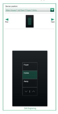
Once the button has been selected and engraved, make sure that the **Program Type** is set to **Normal** and change the **Button Type** (in the upper-middle of the screen) to **Single Action**. **Single Variable** and **Conditional** button types are considered advanced button types and cannot be edited from within the Lutron mobile app, preventing the end user from being able to apply Sonos Room control.
