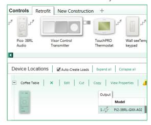
After the Pico Remote Control for Audio has been added to the database, proceed to the **Program** tab of the software and select the Pico Remote Control for Audio from the **Device Location** drop-down list.
