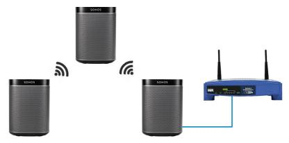
When using Boost Mode, where one Room is wired into the physical network, it is important to limit the number of hard-wired Rooms to one network. Connecting more than one Room to the network using a wired connection could cause a network loop.
