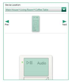
When programming a Pico Remote Control for Audio, ensure that the **On**, **Favorite**, and **Off** buttons are set to **Single Action** button type with **Momentary On When Pressed** LED logic.
